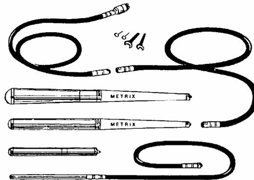
The flexible drive shafts are produced in standard lengths of 3 metres, 5 metres and 6 metres. The flexible shaft for the 281 poker is 28mm diameter and 32mm diameter for the larger pokercs. The versatility of the Metrix system allows 32mm diameter flexible shafts to be connected together to increase overall lengths and also allows 32mm diameter flexible shafts to be connected to a 28mm diameter shaft. Special lengths can be made up to suit individual requirements.
